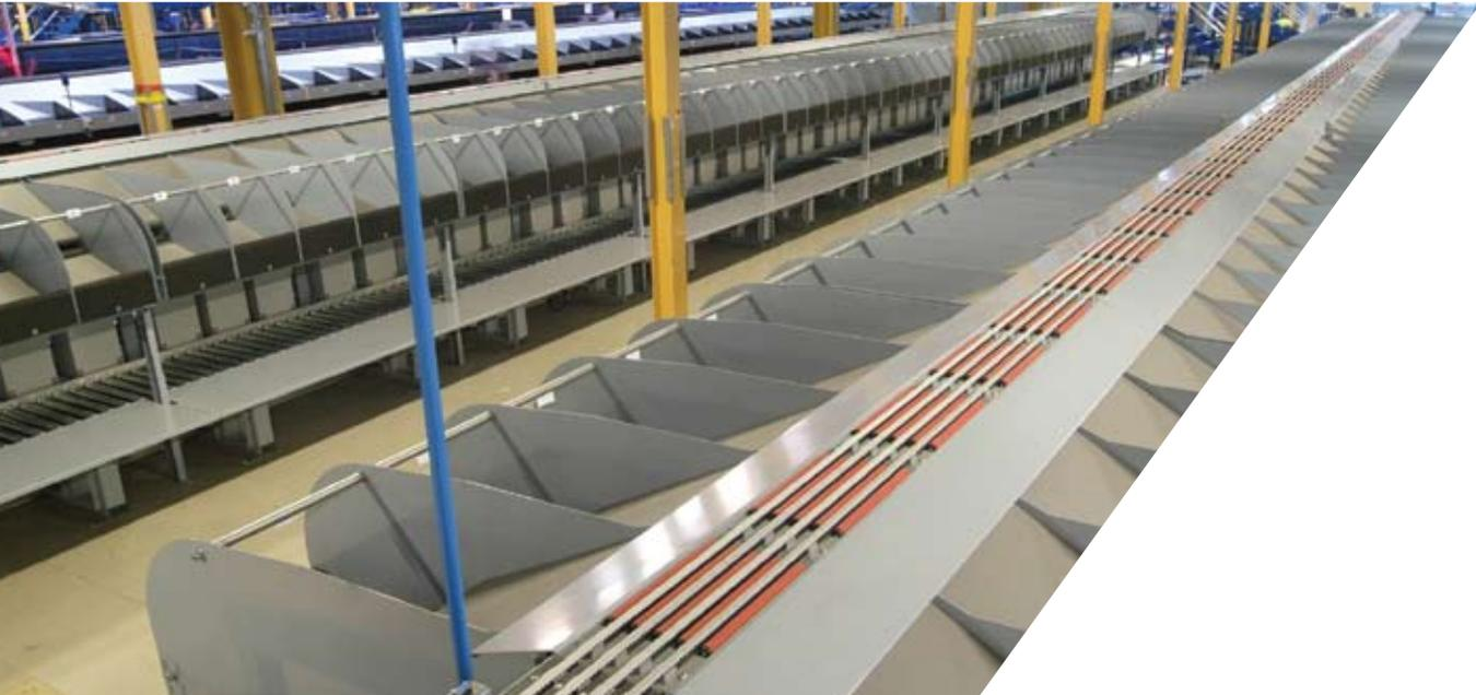
Axiom, the family owned UK manufacturer specialising in the creation of innovative mechanical handling systems, has designed and installed a unique sortation solution into Europe's leading video games retailer, GAME Group plc. The 216 destination pop-up roller sorter has a throughput rated at 20,000 products an hour.
